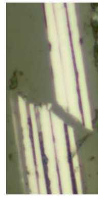
SG 1 /M55 1 /SG 1 Fibre fracture
